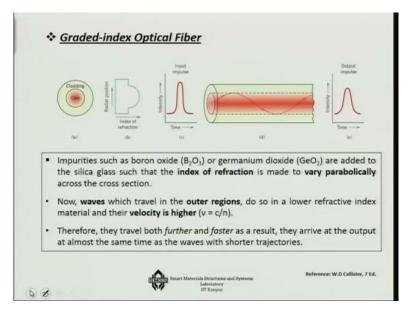
So hence today, slightly more kind of a complex design of optical fiber has come half in which this variation is not stake, but rather in this kind of a form of parabolic variation and this is done with the help of impurities such as boron oxide or germanium dioxide, which are added to the silica glass such that the index of refraction is made to vary parabolically across the cross-section.
