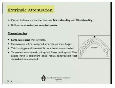
Now what happens in the extrinsic attenuation? There are 2 external mechanisms of extrinsic attenuation; one is called macro-bending and another is called micro-bending, both of them
