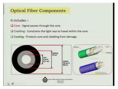
If you look at the optical fiber take a cross-section, you will see that at the very core, there is something which is about 0.8 micrometer to 62.5 diameter of the core that is there, which actually process the signal so that is the core part. Then on top of the core there is the cladding which is about 125 micrometer and on top of the cladding there is a coating which is 250 micrometer to 900 micrometer, so it is a 3 layered structure core, cladding and coating.
