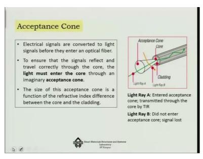
Because the electrical signals are converted to light signals just before they enter the optical fiber, now to ensure that the signals reflect and travel correctly through the core, the light must enter the core through an acceptance cone okay, because if the angle is more than the light will not be able to go inside the system and it will be lost, so it is the function of the refractive index difference between the core and the cladding.
