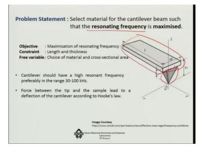
Now, what is the problem statement for us? That select material for the cantilever beam because you see that we are doing it from the resonating frequency point of view okay and we have to maximise the resonating frequency so we have to select material for that probe. This part is very-very small so that is why is not important from the resonating frequency point of view; its contribution to the resonating frequency will be very small.
