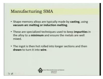
How do we manufacture SMA particularly in the wire form? So SMA are typically 1<sup>st</sup> made by casting using vacuum arc melting or induction melting or similar processes, but both of these processes are highly specialized process and highly expensive process. However, these techniques are used to keep the impurities in the alloy to a minimum and insure that the metals are well mixed.
