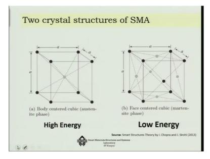
Now the crystal structure point of view, there are 2 crystal structures in SMA one is that high energy or high temperature form and another is that low energy or low temperature form. So it high energy, the form that we encounter is called a Body centered cubic structure Austenite phase okay, so here nickel and titanium atoms as you can see in this system. And in the phase centre, you get it in the phase centered form of the system. Now these are 2 crystal structures, how does it behave?
