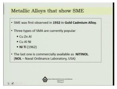
Finally, as the thermoregulation takes place you will see that the same shape is back again. So this effect was 1<sup>st</sup> observed in 1932 in actually gold cadmium alloys. There are 3 types of
