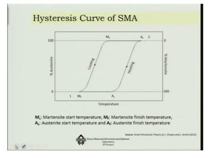
So if I take a SMA wire and if I only change the temperature let us say, so what I will see if there is a way I can continuously monitor that what is happening to the internal material property change, I would see that initially till about say for example, Austenite start point, so I have to go up to this point I would see that the material is that Martinsite formation which is FCC formation.
