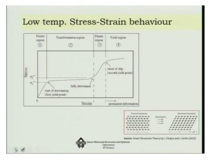
Let us say  $1^{st}$  we consider the low temperature stress-strain behavior. So at the low temperature levels that means at it is at Martinsite, so this is at the Martinsite phase in fact, it is initially at detwinned Martinsite phase. Now as I am increasing the loading, after a certain
