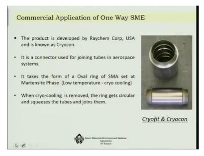
Now, there are many commercial applications of one-way SME for example, this is a Raycherm Corporation product which is known as Cryocon, it is initially a connector which
