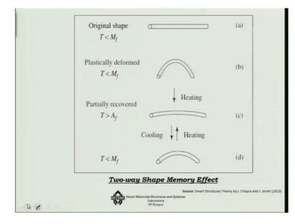
So, how will be the two-way shape memory effect? This is where the original shape at the Martinsite level, you deform the whole thing and then you heat it up, you are going to get this particular shape. Now from this shape you cool it, you are going to go back to this particular shape, bent shape. So now you heat and cool, heat and cool you will be flipping between these 2 shapes, one is at a high temperature memory another is at a low-temperature memory shape.
