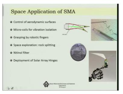
Using this there are many interesting applications that have been developed for example, the control of aerodynamic surfaces like an aircraft wing control, et cetera. As you can see here that SMA wire is controlling this so called angle of aircraft, so that is one application. Micro-
