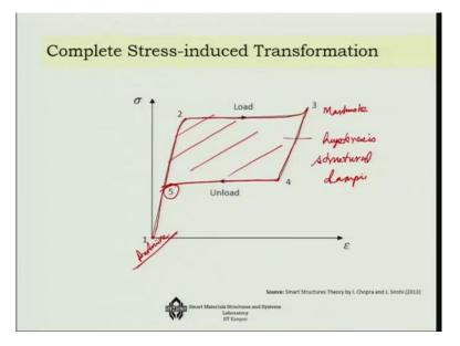
If I look at the pseudo-elastic behavior that means here I am at Austenite phase and then I am increasing the load okay up to 0 point 2, the elastic loading is over suddenly the phase transformation happens, this is stress induced phase transformation and I am going back to the Martinsite phase. And then from that phase I am reducing the load again and then if I reduce it 1<sup>st</sup> initially, it is once again elastic and then the huge change and it comes back to number 5.
