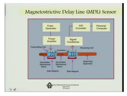
One such typical sensing I am showing you her, which is the magnetostrictive delay line fencing, so what happens is that there is one area where you have applied the magnetostrictive material, you have applied this biased magnetic field which is generating mechanical wave and that mechanical wave is travelling, then at another point you are actually picking up the signal.
