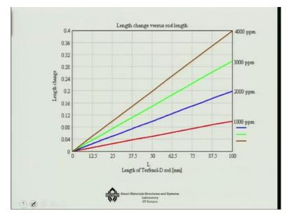
Now, I told you that magnetostrictive materials shows something like 2000 parts per million or little more than that in terms of the strain that tip strain, so how much does it mean in terms of the change in length? So let us say, I choose a 100 millimeters of a beam and I apply these materials over it and then if the full strain if something like 200 parts per million.
