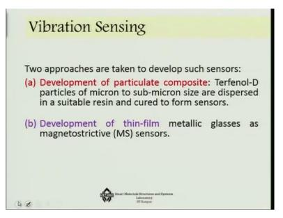
In terms of vibration sensing there are 2 approaches, one is to develop particulate composite like Terfenol-D particles are milt of micron to sub-micron size and are dispersed in a suitable resin and cured to form sensors. And the other one is the development of thin-film met glasses metallic glasses as magnetostrictive sensors, so these are 2 different approaches for developing such sensors.
