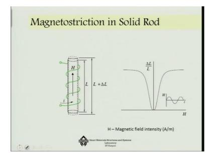
So if I consider a solid rod and if there is a solenoid worn around it, and in that solenoid let us say I am applying a current I, which is going to generate a magnetic field H on the core that you can see here, let that core be magnetostrictive core. Then due to the application of this current, the magnetic field will create an expansion initiate and it will become from L to L plus Delta L.
