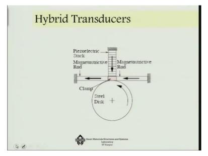
There is something like hybrid transducers also. In this case for example, there is a steel disk okay and this steel disk has clamps here okay and there is a piezo electric stack here so and
