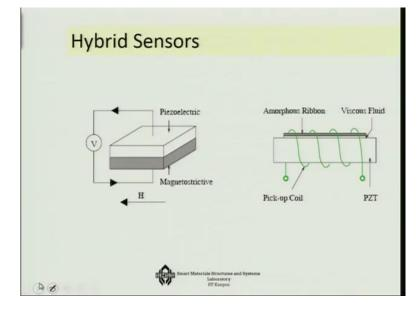
Similarly you can have hybrid sensors like partly piezo electric and partly magnetostrictive. Or you have amorphous ribbon, which is magnetostrictive and then you have pickup coils and also you have the PZTs. So the idea in this type of systems is that magnetostrictive sensor can be used in one part of a strain generation whereas, in the other part you can use piezo electricity thus you can use magnetostrictive material for a large range. (Refer Slide Time: 30:39)
