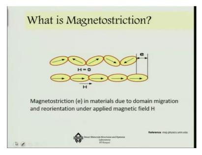
Now, what is the magnetostriction? Magnetostriction material is something which refers to the change in the size of the system due to domain migration and reorientation under applied magnetic field. For example, you consider the 1<sup>st</sup> case where a magnetic material as is always having dipoles magnetic dipole in it and each dipole has its own direction, but these directions are very randomly aligned, so that means in terms of North-South suppose they are very randomly aligned.
