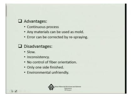
The advantage is this is a continuous process, it is much better than the manual process, faster. Any materials can be used as the mould in this case and error can be corrected very easily by the re-spraying. Disadvantage is it is still slow and there can be inconsistencies, there is no control over the fibre orientation because you are just chopping the fibre and spreading.
