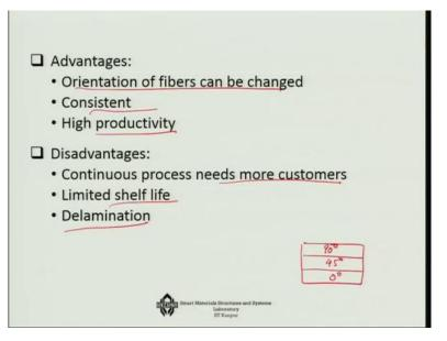
The advantage of Prepreg system is that the orientation of fibres can be suitably changed okay, so in one layer you can have like multiple layers. If I look at the cross-section, I can have multiple layers of multiple direction of ply, so that will be something like 0 degree, 45 degree, 90 degree, I can vary it, so orientation of fibres can be changed. It is consistent and it has a high productivity.
