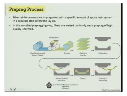
There is another way out which coming up in a good way, it is called a Prepreg process. So here the fibre reinforcements are impregnated with a specific amount of epoxy resin system in a separate step before the layup. So basically you can buy from the market these prepregs. Now in the so-called prepegging step, fibres are actually wetted uniformly and a prepreg of high-quality is formed.
