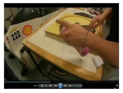
So 1<sup>st</sup> you cleanup this whole space the so-called mould space and then on that mould so you actually apply some release agent so that it comes out very well and then you start to apply the glue and the carbon fibre. As you can see that carbon fibre here is getting applied and this is like it can be of 2 types, one is that you add only fibre or you add carbon fibres like in the prepreg form that means the carbon fibre is already having glues in it.
