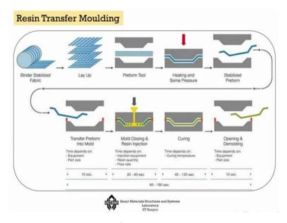
And in this case what we do is that we 1<sup>st</sup> take the fibres okay in a fabric form, you lay it up so that you actually make it of various angles like this is 0 degree and this is 90 degree, again 90 degree, et cetera. And then once you make all these 0 degree, 90 degree layers, then you put it into the preform tool. And once the preform tool you put it, you get it into the shape you like okay.
