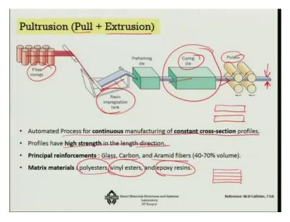
Now there is one way of making actually continuous fully automatic composite laminates and that is called Pultrusion process, which is a mixing of Pulling + Extrusion. So what you do in this process that you take the fibres from the fibre roving and then you can see that they are getting a resin bath here, so this is resin impregnation tank as the fibres are pulled through the tank, they are getting resin bath.
