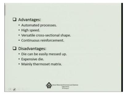
Advantage is that this is an automatic process as you have seen, it is a high-speed process and you can make versatile cross-sectional shapes and continuous reinforcements. Disadvantage is that the die can be easily messed up okay because you are putting it in the die bath and the die can get hardened for example.
