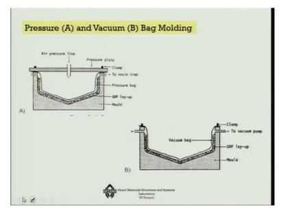
One is Pressure bag moulding; another is the Vacuum bag moulding. In order to improve the fibre volume fraction, suck out the additional resin and make it more compact, you can either use air pressure bagging. So here once you have the mould, you apply the air pressure okay, so you have a pressure plate here, which keeps this whole system into place, apply the air pressure and then there is a resin trap from which the additional resins actually come out of the system.
