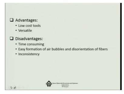
So what is the advantage and disadvantage of this process? Advantage is that it is low cost; you can do it like in a very small set up. It is very versatile, you can make your own mould shape and you can do this. But the disadvantage 1<sup>st</sup> of all is that this is a manual process, so hence it is time-consuming. And when you are doing this applying the resin, there is a these chances of air bubbles getting interact, so easy formation of air bubbles and disorientation of fibre.
