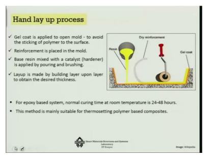
So that reinforcement you then place it to the mould, so that is the yellow part the orange colour part that you have here and then over that you pour the resin, so that is the resin you are just directly feeding the resin. And the base resin is often mixed with the catalyst hardness and so that it gets hardened very fast, so this is the dry reinforcement okay. And ones you are applying the dry reinforcement, over that you are placing the resin.
