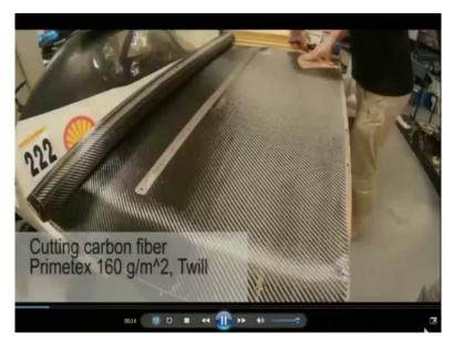
So as you can actually see in this particular case that 1<sup>st</sup> of all you are cutting the carbon fibre and of particular shape that you want to do. In this case, they wanted to make a circular shape, but instead of making the whole circular shape they are cutting it into various pieces like 6 to 8 pieces okay and that help can be developed in terms of layers. (Refer Slide Time: 18:19)
