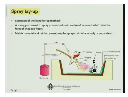
Slightly better technique is the Spray lay-up technique, so this is an extension of the hand layup. And in this case instead, of pouring the resin, what you basically do is that you take a resin supply through a chamber pipeline and there is a catalyst that is coming, so these 2 are getting mixed here and then the resin is coming out. Not only that, many a times what we do is that the fibres also like using a chauffeur gun many a time we also split the fibres through the same process.
