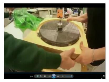
So thus they have done it, after this they have to put it for curing so they are just opening up the vacuum bag and taking the whole system out, the carbon fibre reinforced system and then you need to cure it. Now in some cases they put it in auto club where the both the pressure and temperature is applied and in some cases they only apply temperature and cure it.
