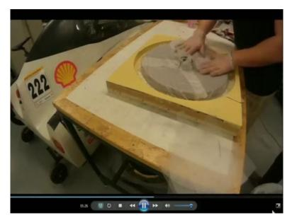
Now once the required number of carbon fibres you have applied, then what they are doing is that they are applying this white film which is the release films, so that it comes out very easily and also the bigger you have to apply so that it gets cured very easily. And then you have to apply the vacuum bagging, so basically they put the entire thing into the vacuum bagging system, just now we have discussed about the vacuum bagging.
