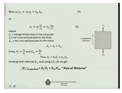
We see that Sigma c A c = Sigma f A f + Sigma m A m, which means Sigma c = Sigma f A f by A c + Sigma m A m by A c. And since you are considering the cross-sectional area and you consider the unique thickness of the system, so in this direction okay, so consider a unit thickness, so this is really thick. Then A c you can say it to be A f + A n and that is nothing what V f and V m, so hence Sigma c = Sigma f V f + Sigma m V m.
