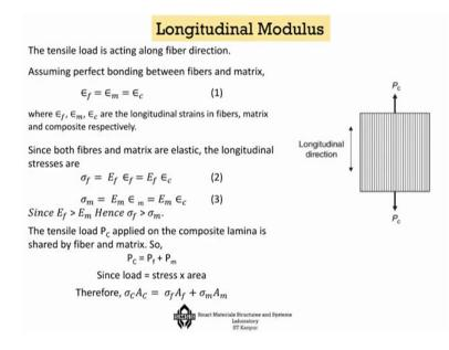
For example, if I consider the longitudinally modulus, then if you assume perfect bonding between fibre and the matrix, then the strain in the fibre equals to the strain in the matrix that is strain in the composite. In this case longitudinally modulus, you are having fibres and matrix as if there are two different springs which are in parallel. So something like I can show it to you through this particular example.
