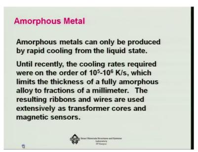
Now can metal not have an amorphous shape that is, can we not have metals which has no regular crystal structure? Yes we can, but to do that you have to have a rapid cooling from the liquid state. Now, until recently the cooling rate required is of the order of 10 to the power 5 to 10 to the power 6 Kelvin per second so, so fast you are supposed to cool it if you want to really make a metal amorphous.
