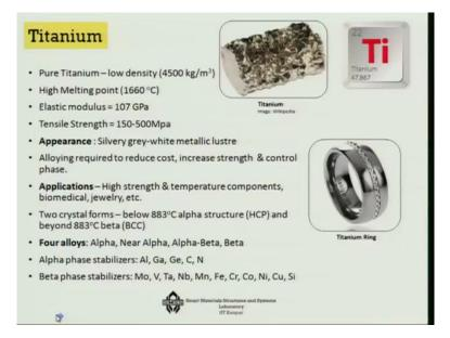
Now, the next thing that became important in terms of transport applications is actually Titanium. Its density is actually higher than Aluminium but lower than Steel, so we always say in a density scale density of Aluminium is actually less than the density of Titanium and density of Titanium is less than the density of Iron based alloys. So it is about 4500 KG per meter cube, its melting point is quite high 1660.
