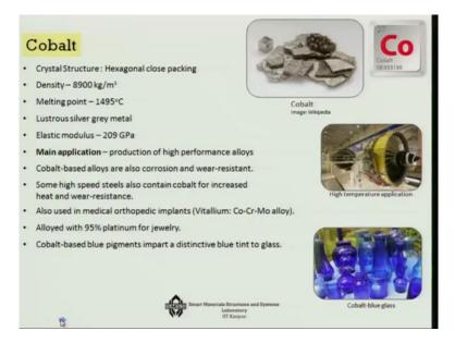
So Cobalt already we have seen that it is used for example with Steel as an alloy or also with other metals, but on its own Cobalt has had the Hexagonal close packing HCP. Density similar to Nickel 8900, melting point also is very high and the lustre is silver grey, elastic modulus is about 209 gigapascal consider about like Steel, main application is for high performance alloys particularly when just like Nickel and Zinc you need a corrosion and wear resistance, the Cobalt comes into picture.
