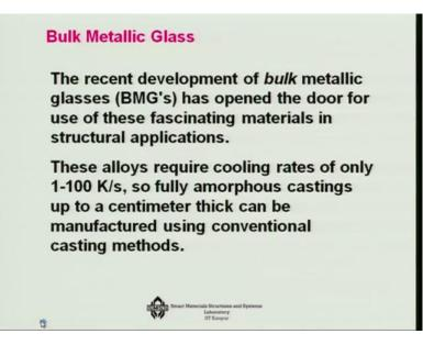
Now the bulk metallic glass is something which its cooling rate is bought down to something like 1 to 100 Kelvin per second and that is possible because of some kind of eutectic mixture that you are that today we can do for preparing this. For example, you can see that this is a Bulk Metallic Glass structure and you can see that in the same picture that there is no grain okay unlike this polycrystalline metal structure, where you can see that so many grain boundaries of there.
