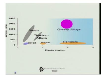
So in this last picture if you look at it that in terms of strength if you can make the glassy alloys, you are going much higher above the Steel that is where the advantage of the glassy alloys is. And if you look at the percentage strain also, you can go much higher above the Steel Aluminium, et cetera, something like which we can compare only with polymers.
