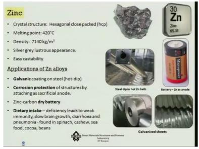
The next is Zinc, now Zinc shares one commonality with Titanium is that this is also Hexagonally close packed HCP, but its density is very high. We are suddenly now jumping from a low-density to a reasonably high density very close to Iron, 7140. Melting point is also not very high, 420 degrees centigrade; it has a silvery grey lustrous appearance and easy castability.
