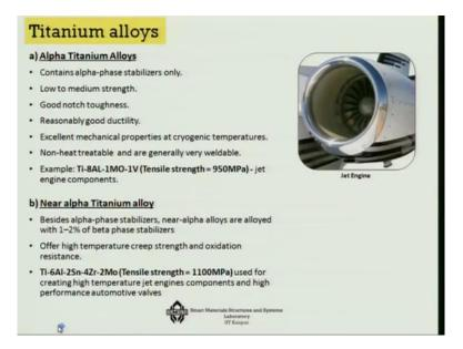
Now titanium alloys, let us talk about a little bit of them Alpha Titanium alloy to begin with that is the low-temperature phase. It contains the Alpha phase stabilizers, low to medium strength; it has good notch toughness, reasonably good ductility, and excellent mechanical properties at cryogenic temperature, but it is non-heat treatable that is the problem with Alpha series and is generally very much weldable.
