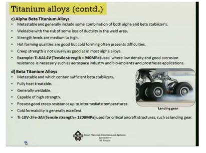
Then you have the Alpha-Beta, this one is metastable that means it is not very much stable configuration, generally includes some combination of both Alpha and Beta stabilizers. It is weldable, but if you weld there is risk of loss of some amount of ductility, Strength levels are medium to high, hot forming qualities are good but cold forming often represents difficulties. Creep strength is not usually as good as in most Alpha alloys.
