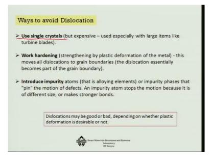
If you use a single crystal structure, generally to do that you actually control the environment to a very good degree, you can avoid the dislocation for example, turbine blade making this is done, but it is very expensive okay, so that is why it is not usually done. The other way to do is actually work hardening. Now because dislocations are happening inside the grain structure okay, so you what you can do is that through work hardening you can move all the dislocations to the grain boundaries.
