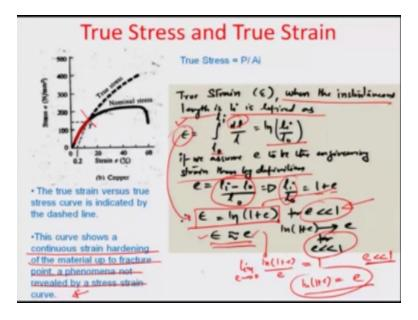
So similarly you can actually have true strain when the instantaneous length is Li from an original length Lo you can define the strain as the change in length dl per unit l and integrating
