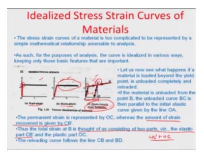
There are many materials which can be idealized in terms of their stresses and strains. For example, let us say if there is a rigid plastic or an elastic plastic or elastic linearly strain hardening material these are the strain curves stress-strain curves you know which represents the various ideal situations so for example in a rigid plastic gate there is a there is a ultimate stress
