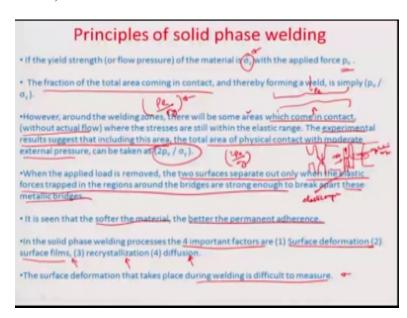
So let us look at the series of events which happen in such processes so if we consider the  $\sigma_y$  to be the bulk strength of the material or it is the yield strength of the material and we apply a force
