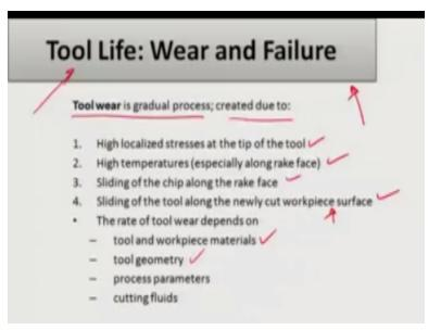
The other issue which I wanted to really emphasize is that because of all these temperature rise and you know severe plastic deformation of the chip material formulation of built up edge there is an effect on the tool life you know particularly because of the wear and failure in many cases of the tool or in some cases sort of a protect length layer which happens because of which the tool I may increase okay.
