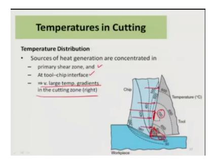
So if I look at the various temperature distributions which have been found out in the primary zone the tool chip interface you can see that you know there are very large temperature gradients particularly in the cutting zone if you look at the gradient here for example the temperature line the isotherm here which is recording hundred and thirty degree Celsius is just closely spaced to the two temperature which is about 500 degree Celsius.
