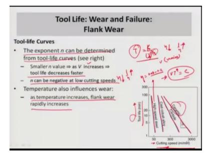
Extending this logic further the tool life curves can be plotted for different values of n the exponent n can be determined from the tool life curves really you can see here you already know that C/V or some constant K which is C  $^{1/n}/V^{1/n}$  = tool like T obviously if n is a smaller value and 1/n is quite large then if V varies let us say V increases or V just varies so for a larger coefficient here the tool life should be able to vary more.
