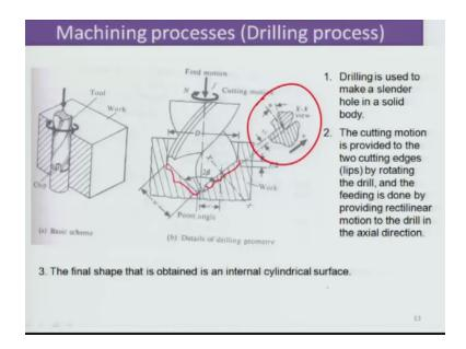
Having said that, let us now actually start looking into the mechanist aspects of drilling. In this particular case as well you can see that there is a peeling motion which is happening here by the two edges at the end of the drilling cutter and there a peeling action happening as you can see which is similar to that is happening to all the other different processes like milling or lathe or shaping, planning etc. in the same peeling action.
