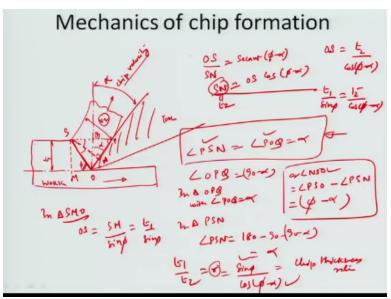
So I will just relate the figure a little bit or the sake of understanding. So you see then again the same point SONP and Q is now this point is here right about here, right about here is the vertical intersecting with the perpendicular projection of the point S on to the tool surface okay. And the shear angle here is  $\Phi$  for example, this is N point where the perpendicular form has tool surface again and that is how the geometry is okay.
