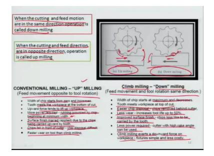
We also wanted to see about the different of kind of milling operations which are there in that context we are done earlier and we had seen a various orientation of the tool with respect to the work piece in case of slab milling, slot milling, form milling, face milling and milling so and so forth. So typically you can classify also the milling processes into up milling and down milling these are different illustration of happens.
