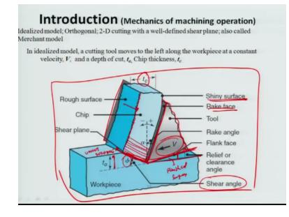
So let us now finally get into studying of this peeling action which is going on here right about expressed in this particular figure. So this is the uncut surface and you have a tool point or a tool tip which is actually a single point tip though, but then there is a cutting edge which is associated with this. And it moves with respect to the work piece in directional which are parallel to the direction of the movement of the work piece.
