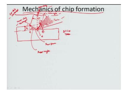
And if time permits we will do some oblique angle but by largely will focus on to this orthogonal cutting operations related to mostly used form of cutting within the industry. So let us look at the geometry aspects of how chip gets formulated. So you have a work piece here and you have a chipping process which happens in this particular zone right about here, due to which there is a formulation of finished surface which comes up.
