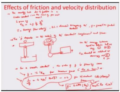
So the energy loss due to friction in a circular conduit and these are some of the assumptions were borrowing from elementary fluid mechanics and basically the more important part that has to be seen here is the application that how these energy loss is going to change the time of filling etcetera related to the cast so I am not going to actually prove the how the loss balance equation or how the energy loss balances happens for a circular conduit for a laminar or a turbulent flow case.
