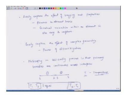
In reality here just for the purposes of explaining I have said that there is a small gap but in reality because nodes 2 and 3 are at the same physically at the same location then there is no reason to think that the temperature of t2 will be different than temperature of t3, so we will ensure while we are doing assembly that the temp, value of temperature t2 the same as the temperature at t3. So these 4 equations will merge and then we will lose one equation in that process.
