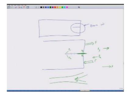
If it is not continuous then we do not do that. In that case we do something different for instance here if there is no friction on the interface boundary then we say that there is no shear force there is no shear force at the location p, p3 so that maybe the other condition so that is the extra condition we impose in case of fracture for this particular kind of problem.
