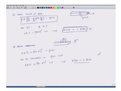
Axial motion of the bar and beam vibrations, it turns out that  $\lambda$  represents the angular frequency square of angular frequency okay, that is what it turns out. But now we will consider case where?
