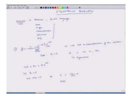
Another example so, so before I go to another example here the governing equation is  $m\ddot{x}+kx$  is equal  $F_0$   $e^{i\omega t}$  okay, and if  $F_0$  is equal to 0 if  $F_0$  equals 0 then my equation becomes  $m\ddot{x}+k_x$  equals 0 or I can express it as  $\ddot{x}$  equals minus k over m times x or I can write this as a function of x which is the right side equals.
