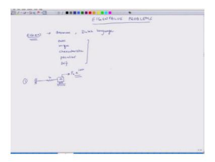
So I will give you an example, first example so I have a spring, mass and I apply a force and let us say I apply a harmonic force  $e^{i\omega t}$  okay. Now when I am exciting it with this force, when I am exciting this system with this force whose frequency is  $\omega$  then the system will get excited at the same frequency  $\omega$  so this  $\omega$ .
