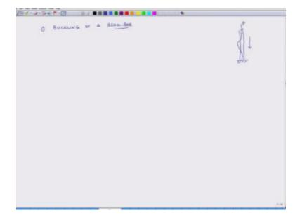
The bar will do this, so it will buckle when the compressive force P exceeds a particular number, that particular number depends on the characteristic of the system it does not depend on P, so this is one case where the Eigenvalue is not related to the.
