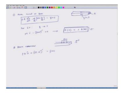
But right now we will discuss beam vibrations okay, so for a beam which is a cross section A and a moment of inertia I and Young's modulus e and density is  $\rho$  the governing differential equation, the dynamic dynamical equation is the  $\rho A$   $\ddot{w}$ , second derivative of W, so W is reflection plus EI(w") equals f, f is the distributed force on the beam, again if I have to find the Eigenvalue of this system the first step I have to do is I have to, I have to equate.
