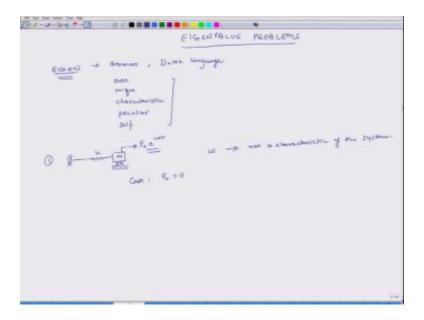
Is not a characteristic of the system okay, but suppose I remove this force, so case when  $F_0$  is equal to 0, and then if I disturb this mass by a little amount then the system will vibrate back and forth at a unique frequency. Let us call that unique frequency as  $\omega$ .
