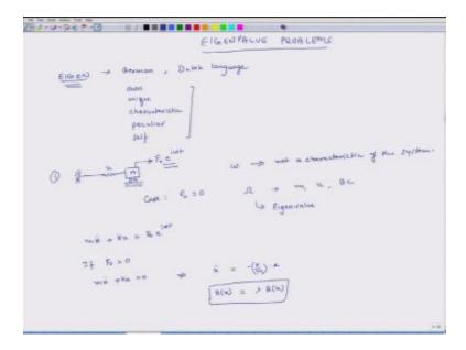
Some constant  $\lambda$  and this  $\lambda$  maybe an Eigenvalue, so if it, so sorry before I use that, times another function of x which is B(x), so if I can express so if there is a system which does not have which is not seeing any external force and if I can represent that system as.
