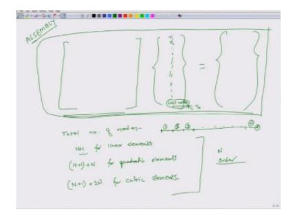
That temperature, that outside radius is  $T_o$  okay. So I go to my assembly and  $T_o$  will correspond to the last node right, and this is a column of all the temperatures right. This is  $T_1$  first node  $T_2$  and whatever is n+1 nodes for linear elements or 2N+1 for quardratically so this is the last node. So I say okay I will put in this vector it will not be unknown now it is known and its value is  $T_0$  its value is  $T_0$ .
