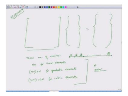
Then you do the assembly then the total size of your metrics will be N+1 for linear (N+1)+N4 quadratic and so on and so forth. So this is by assembly process, so once we have done the assembly I have captured the whole geometry of the system in my equations. We have started from R is equal to  $R_i$  to R is equal to  $R_0$ , pura  $\sqrt[4]{R}$  geometry capture kiya  $\sqrt[4]{R}$ , also I have captured.
