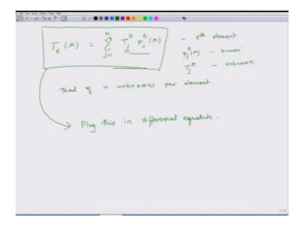
We have to find n unknowns per element, if we choose a linear element then we have to calculate two unknowns. If we choose a quadratic element we have to find the values of n points and also add one middle point. If we have to, if we choose cubic element we have to find four unknowns and so on and so forth right. But the point is that we have assumed that this is how T varies over radius.
