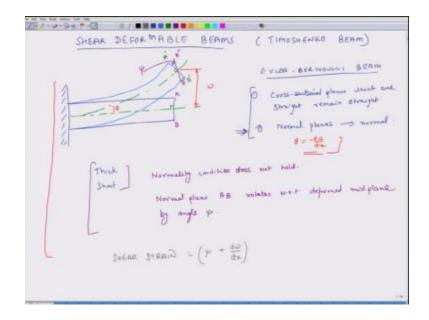
This is that not only we get to learn a little bit more about beams, but also because of the fact that in this particular case when we create our stiffness matrix we have to resort to some different methods which are known as reduced integration methods when we are computing the stiffness matrix, so I wanted you to become aware of these methods also as you get deeper into finite element analysis. (Refer Slide Time: 10:50)
