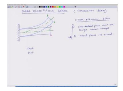
And these are also known as Timoshenko beams, and the theory which describes this particular beam is known as Timoshenko beam theory. So first let us recap what is an Euler beam, so suppose I have a straight beam and let us say this is a cantilever, so it is rigidly fixed at one end and when I apply a force then this beam bends and the light blue color depicts the bent shape of this beam.
