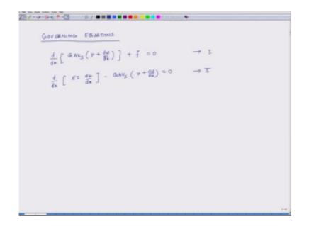
d over dx,  $GAK_s$  times  $\psi$  plus dw over dx plus f equals zero, and the second differential equation is EI d $\psi$  over dx minus  $GAK_s \psi$  plus dw over dx equals zero okay. So this equation the first one relates to the equilibrium of forces and the second equation relates to equilibrium of moments okay. So first one ensures the w direction degree of freedom has equilibrium, and in the second case the rotational degree of freedom is addressed. (Refer Slide Time: 12:57)
