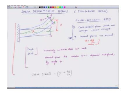
Detail about a typical shear deformable beam, and in this case the shear strain is equal to  $\psi$  + dw over dx that is the shear strain, so with this background what we will do is, we will now develop a finite element formulation for this type of a beam, and the reason I am doing.
