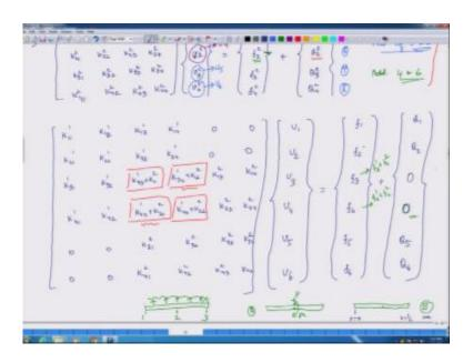
If that is the extreme end of the beam, then in our equation  $Q_5$  and  $Q_6$  will be prescribed as zero,  $Q_5$  is the shear force and  $Q_6$  is the moment okay.
