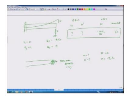
Likewise, I have another boundary condition, and it is that when it is bending I have a torsional stiffness,  $k_T$ , in this case the moment in this you know this is a torsional spring, in this case again w is unknown w' is unknown shear force, I am not putting explicitly any shear force so that is zero. But moment is equal to what? Rotation which is  $u_6$  times  $k_T$ , and it opposes the rotation so it is minus. So suppose the torsional stiffness is  $k_T$  then this is here okay.
