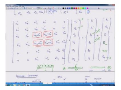
So we go back and again put these modified boundary conditions, so  $u_1$  we said is 0 because it is clammed and  $u_2$  is zero, because it is clammed in and moment was 0, and this we specify as minus K times  $u_5$  okay. Now when I solve this equation I have to move.
