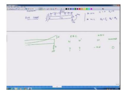
And that is suppose you have a spring at the end, then what will be the condition at the boundary condition? So in this case our natural essential boundary conditions and then we have natural boundary conditions right, so this is our shear force and this is our moment. So w is known or unknown, w is unknown right, we do not know what is w, we do not know also the slope, we know that moment at the end is 0, there is no moment being prescribed.
