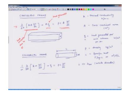
Now all these equations they do not account for convective heat transfer so for instance if you have this bar it could be surrounded by here right, and there may be not only heat transfer due to conduction but also because of conviction so he here will pick up some heat and it will that heat will get disputed into to here so here we do not have a convective term in this entire equation.
