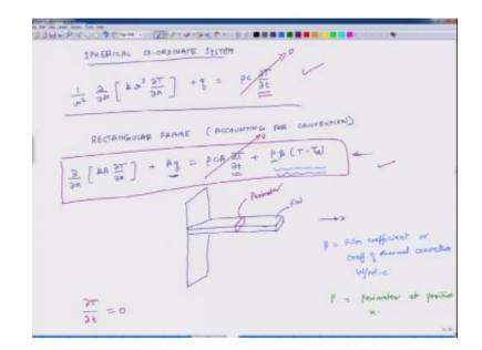
And this equation they all have this partial of temperature with respective time so this is for a system where we are looking for transient solutions, where solution is changing with respective time if the solution does not change it time then it will be a steady state system and steady-state system partial of temperature with respective time will be 0, so in this case this term goes to 0 for a spherical coordinate system this term goes to 0.
