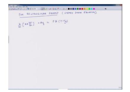
So for , for rectangular frame okay my governing equation steady state equation the governing equation is partial with respective x KA  $\partial T$  over  $\partial x + Aq = P\beta$  times  $T - T_{\infty}$  by the way I did not explain what is  $T_{\infty}$ .
