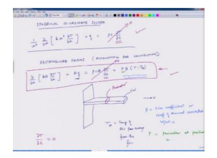
So in this case  $T_{\infty}$  is the temperature of surrounding here so it is temperature of air and it is infinity because we are measuring this temperature quite far away from the FIN temperature of air far away from the FIN So that is my  $T_{\infty}$  if  $T_{\infty}$  is small then we will have more convective heat transfer if it is more than convective effects will be less and  $\beta$  is I explain it, it is film coefficient.
