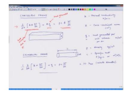
For heat conduction with respect to different farms of references, so if we have a Cartesian frame of reference then the 1D equation and this we have seen it earlier also is kA  $\partial T$  over  $\partial X + Aq = \rho$  CA  $\partial T$  over partial of temperature with respect time and K is thermal conductivity and it is units of are w/m-d centigrade then A is cross-sectional area so to give you a context suppose I have a some bar then the cross-sectional area of this bar represents A
