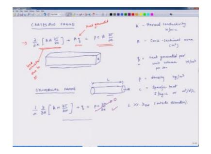
For a cylindrical frame of reference this term goes to 0 so if I just drop the temperature derivative of the time derivative of temperature then I can get steady state equations.
