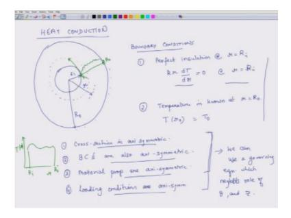
We are trying to calculate how is temperature, see here  $r=R_i$  and here  $r=R_O$  here  $r=R_i$  how is temperature, so temperature varying, it could vary this readily in the radial direction, so this is so I am trying to make a plot, x axis of the plot represents radius, y axis represents temperature, so I am trying to get a plot of this nature, this is radius, this is temperature as a function of r and the domain is  $R_i$  to  $R_o$ , inner radius to outer radius okay.
