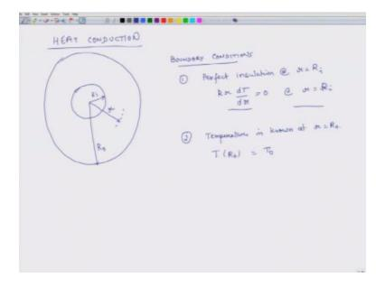
So, so what we will do is consider the example of heat conduction okay, so suppose I have a hollow pipe and this is the outside diameter, outside circle, the inside circle is having a radius of  $R_i$  and the outside circle has a radius of  $R_o$  and at some radius it is R. So you have a hollow pipe so what essentially you are seeing is the cross section of the pipe, and let us look at the boundary conditions.
