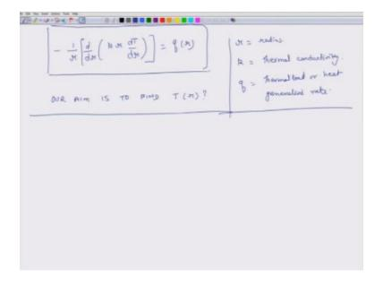
So the governing equation for this problem is this, and our aim is to find T as a function of r okay, so what we are interested in finding out is how does T change as I move from  $R_i$  to  $R_0$  from inside radius to outside radius, that is what my aim is okay, so.
