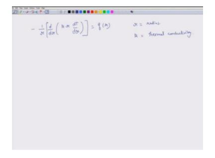
Heat conduction problem steady state heat conduction problem the governing equation is 1/r [d / dr ( k times r dT) over dr] is equal to q(r) and I will explain that, so here r is the radius so if I want to calculate the value of temperature at radius R that is what it means okay, k is thermal conductivity and this thermal conductivity does not change with  $\theta$  direction but it can change in the radial direction that is why.
