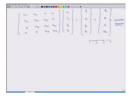
So, we will rewrite the global equation so  $K_{11}$ ,  $K_{12}$  0, 0, this term should be zero, multiplied by global degrees of freedom. Now, what we see is that in our original problem statement we had broken the domain into three elements right. Node 1, node 2 node 3, node 4, so there are four degrees of freedom, because each degrees each node is associated with one unknown which is u, so there are four degrees of freedom, and we have four equations, so this is the first thing.
