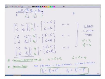
Then the same thing would hold, there temperature of node two for the first element would be same as temperature of node one of the second element okay. So first thing is that we write down these equalities, so these are known as continuity conditions. Continuity conditions for primary variable, we assume that throughout the domain of the problem the primary variable which in this case is u is continuous.
