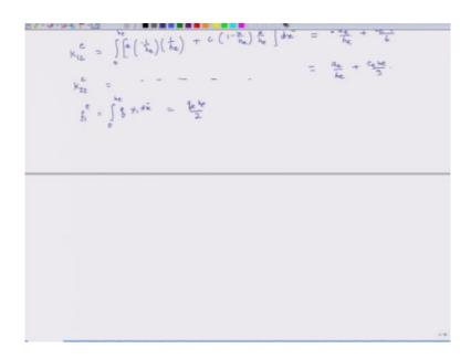
$f_1^e$  is equal to integral of q times  $\psi_1$  d $\bar{x}$  0 to  $h_e$  and if I do the math what I get is  $q_e$   $h_e$  over 2 and  $f_2^e$  is also  $q_e$   $h_e$  over 2.
