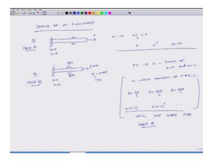
What does that mean, suppose I have a bar and I am pulling it and I am also applying some traction on this, x at x=0, u=0 right. Then when I am making a choice for weight function, I have to ensure that w is zero at x=0 okay. What could be an example of such a weight function, one example could be x, another example could be  $x^2$ , another example could be x and so on and so forth okay.
