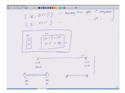
So in this case, bending moment is known at both ends and because I am not applying any vertical sheer force, so sheer force is also known. So in this case, both at both ends I know the natural boundary conditions, and in the third case which may be something like this, I may have a mixture of some essential boundary conditions are known and some natural boundary conditions are known okay.
