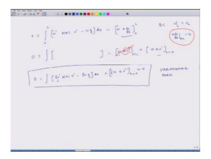
So my original governing equation was this weak form, this is the original weak form of the, for the system right, and my boundary condition was u at zero is equal to some constant  $u_0$  and a du over dx at x is equal to L is zero okay. So what I can do is I get the same term here, [-w au'] where x = L, and  $+[w \ au'] \ x=0$  okay, so what I have done is I have just expanded this term in the parentheses.
