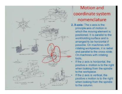
So, we were talking about the different directions used in nomenclature for NC machining and I have just made you exercise, how to figure out the z motion in a for example, rotating work piece system or a rotating tool system. In that we had considered two operations, one is the face milling operation and another is normal lathe based, you know turning operation.
