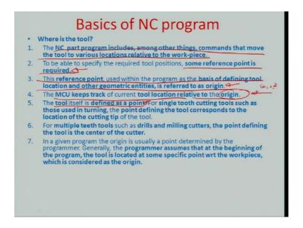
So, the NC part program includes among other things commands that move the tool to various locations are related to the work piece and so for that movement; obviously, there is the requirement of some reference point, which can be considered as a origin or as a start point to start the positioning with respect to. So, it is basically the origin of the orthogonal coordinate system, in which the part drawing has been layout in that particular manner.
