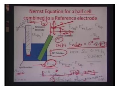
So, let say we are just trying to connect these two electrodes externally using voltage measuring device. So, in that case the E cell in this particular configuration can be written
