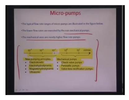
Let us look at some of the comparative flow rates of these micro pumps as illustrated in the figure below here, typically mechanical ones are the most flow rate ones, you have a higher
