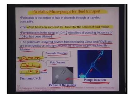
So, this right here is the example of what peristaltic pump would typically do for fluid transport. So, let me just rerate peristaltic is in the motion of a traveling contractor or fluid
