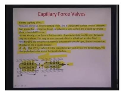
So, you can call it several other names like electro wetting effect and essentially it happens, because the surface tension essentially changes between two immiscible conductive liquids between in a sold surface and liquid just by varying the potential difference between these. So, here as you are seeing this is a uniformly distributed bubble with double layer across at you have some positive charge coming here, some negative charges outside this bubble here.
