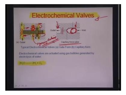
So, let us see what electrochemical valves really are essentially a very simple system of a reaction as can be seen here  $H_2O$  is electro chemically converted in to hydrogen and oxygen. And basically if you look at the overall architecture of these systems this is basically the outlet of micro pipe and this is a gating device here. And essentially there are four electrodes
