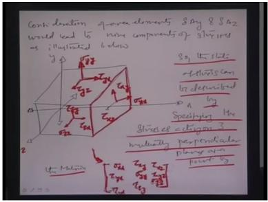
say plane point into the x direction applying point to the y direction and the plane pointing to a z direction in a rectangular coordinate system.
