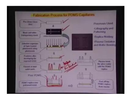
So, the way you make this devices using fabrication strategies for micro fabricated PDMS glass capillaries and the following manner you take a mask here and essentially you pre-clean in a glass slide and then spin coat some photoresist material and expose selectively using this black and white transparency mask. So, that you can actually create these features on the photoresist material, this is the negative tone water resist may be as you wait obtain from a company called Microchem.
