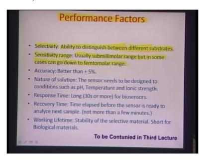
So, the next aspect in sensor design which comes very often is at the end of the day we have to ask the sensor to do a job and whenever it comes to doing a job there have to be measures and beings to identify whether it is doing extra efficiently and so for that there are several aspects which one needs to consider for understanding, you know the performance of particular sensor for trying to take up an analyte. So, this classifies under this performance factors.
