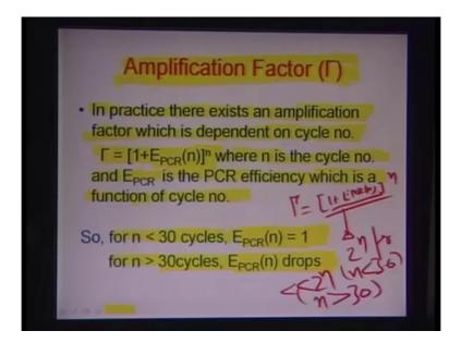
So, there is a important factor here call the amplification factor gamma which is of some importance in practice their existence simplification factor, which is also dependent on the cycle member. So, normal is 2 to the power n. So, amplification efficiency should be one. So,
