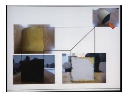
Second object, the front view, the top view, the right side view and if you correlate different features of these objects in different views, this is how your projection lines are going to show up in your drawing.
