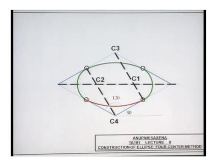
Now, this edge of the rhombus is at 30 degrees to its horizontal this is 120 degrees same thing draw the longest diagonal first from here join the midpoint from here join or rather from here join the midpoint. We will get the centers as c 1, c 2, c 3, c 4, you know the construction you can go ahead you know construct this proximate ellipse not a problem.
