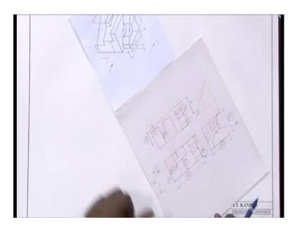
Let me now start sketching the object, remember that I am drawing this in the third angle autographic projection. So, if I view the object along this direction, what will I be seeing, I will be seeing the bottom edge, so if I look at this object in the frontal plane, which features of the object will I be seeing. So, I will be seeing this line all the way through from here to here and then from here to here, now this entire dimension from this point up till this point is 90 millimeters.
