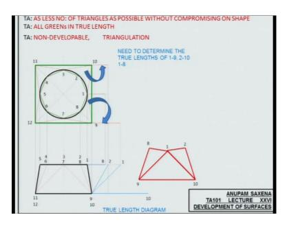
This is another very interesting solid. The front view given the top view given, this cross section is circular, this cross section is rectangular or square. So, this surface is actually a blend between the circular cross section and a rectangular cross sections. Can you imagine this?
