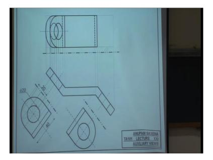
So, this is the front view of the object; this is the auxiliary plane one, auxiliary plane two, and looks like I will able to show the two shape only in or only using auxiliary plane not
