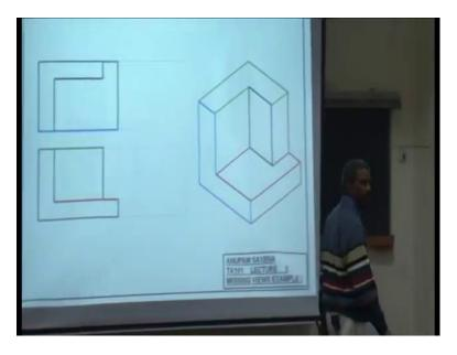
So, this is loop that you see in the top view this guy here this is the loop that you see again in top view this the loop the l loop that you see in the front view. Then, you see a rectangular loop again in the view and now the problem is just to place t is loops appropriately in 3 D had you do that let us see.
