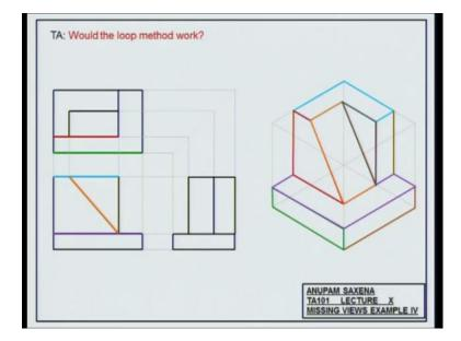
You see the First loop here trapezium second loop rectangle third loop at the top fourth loop again at the top and then you have this rectangular loop at the top and you have this triangular loop on the front. In the front, the purple loop has to go where here the red loop has to go where the green loop stay there the brown loop would it stay like that would it change in shape like the sky blue loop stays there the black loop here.
