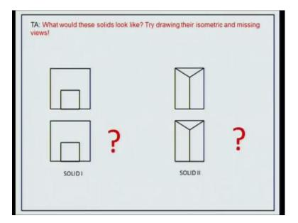
Top view of solid two they are identical to each other and the other time it does not matter if we using first angle scheme or third angle scheme since they are identical to each other. In both cases, in both cases try to find how the respective solid will look like number one and once you do that try to find the missing profile view.
