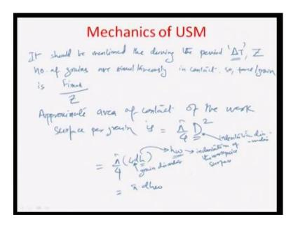
So, let us actually try and do that by looking at, what is the force at least per grain, which comes between the several grains which are there, it mean I said the tool and the work piece surface. So, it should be mentioned that, during the period delta small t or delta capital T where the indentation is happening. It is not a single grain, which is doing this indentation. So, if you assume that, there are z grains which are they are between the tool and the work piece surface.
