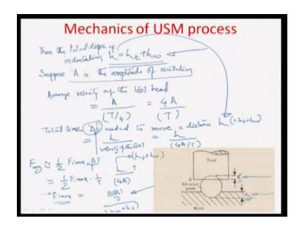
And therefore, one thing is very clear that, because there is a depth of indentation both on the tools side and the work piece side. In this case, for sake of convenience we are representing it by h t and h w. So, the total depth of indentation, h as represented by h t plus h w, where obviously h w is the work piece indentation and h t is the tool indentation, from the tools side. Supposing, A is the amplitude of oscillations, actually it predicts the motion, the philosophy of the tool.
