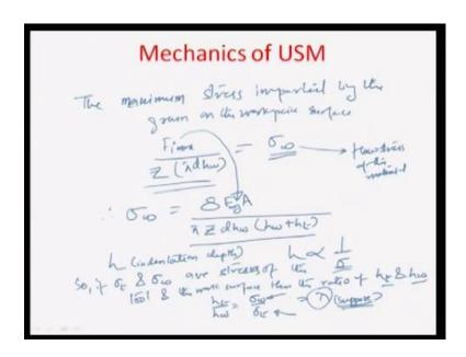
Simultaneously, the maximum stress imparted by the grain on the work piece surface is
