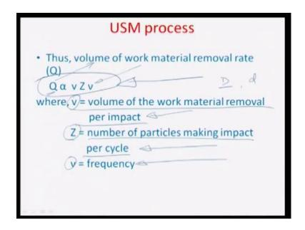
And if you really go for a predictor estimation of the MRR or the Material Removal Rate of a USM process, this actually comes out to be of the form Q proportionate to v Z nu, where v is the volume of the work material removal per impact. And we will calculate this. What this volume is, in terms of indentation? Z here is the number of particles making impact per cycle. So, this basically at one impact, how many particles are coming between the tool head and the work piece surface?
