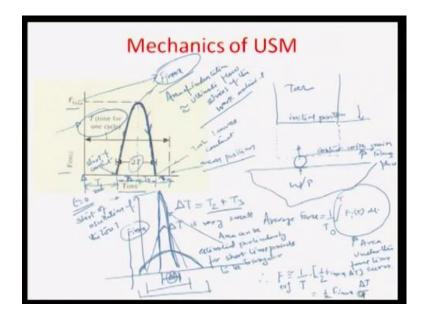
So, if we really look at the variation of the force F i with respect to time, it looks something like this. So, as you can see here, is a several stages in the plot, where the whole grain is being hammered and crushed between the tool and the work piece surface. You start with time t equal to 0 here, for example. So, this is the case when the grain the abrasive grain is free. There is no direct contact of the tool of the grain.
