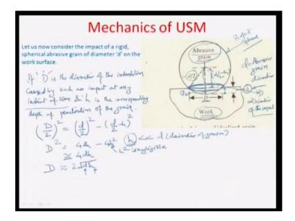
So, let us look at a little bit further by assuming that, in a USM process, now this is the work piece. And there is an abrasive grain, which is hitting the work piece. It is coming down, as if it is plowing the work piece. And we assumed that, there are two different diameters in questions. One is small d. As you can see here, the small d is nothing but, the diameter of the grain. So, it is the abrasive grain diameter.
