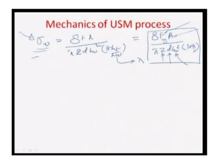
So, therefore the maximum the sigma w, the ultimate hill stress which is develop can slightly be modified as 8 F A divided by pi Z t h w square times of 1 plus h t by h w, which actually signifying this constant lamda. So, we can write this down as 8 F A divided by pi Z t h w square by 1 plus lamda. So, as of now we will continue this in the next lecture.
