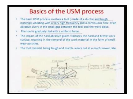
The USM basically is a process again which involves a vibrating tool head. And this was illustrated yesterday, very clearly. And this tool head is basically used over an abrasive slurry. You can see, this is the region of the slurry. This is the work piece. This right here is the tool. And so basically, small amplitudes of motion about 15 to 20 microns are given to this tool head. And it quizzes or compresses the abrasive particles, which are coming between the tool and the work piece.
