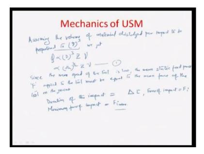
So, let us assume that and let say that the volume. So, we assume here, the volume of material dislarged per impact to be proportional to the cube of this diameter. So, we get the Q from the Shaw's theory earlier is proportional to volume of the work material removal per impact, which is actually cube of this D. For obvious reasons discussed before, times of the number of grains or a number of particles coming to, deliver the impact per cycle, and so the cyclic frequency nu.
