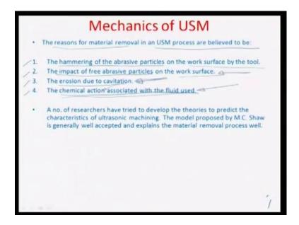
So, this right here of material removal in the USM process. And the principle reasons for material removal, a kind of illustrated here in to this four categories. And the first category is, because of the hammering, a direct hammering of the abrasive particles on the work surface by the tool. The second category is the impact of free abrasive particles on the work surface. So, what you mean by free abrasive grains here?
