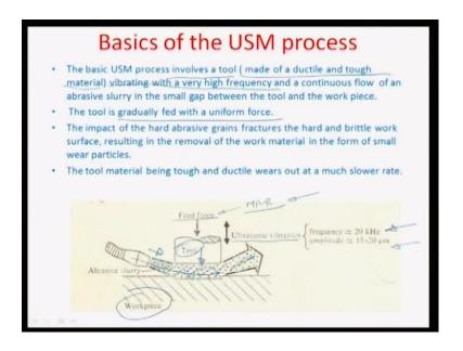
So, this is how the process looks like: you have a tool head which comes in strikes, on the slurry. The slurry is moved between the work piece and the tool head at a certain rate and the slurry typically, can contain mixture of a abrasives and water and this tool had forces down at a certain frequency and the squeezes, the abrasive grain against the work piece thus causing brittle fracture.
