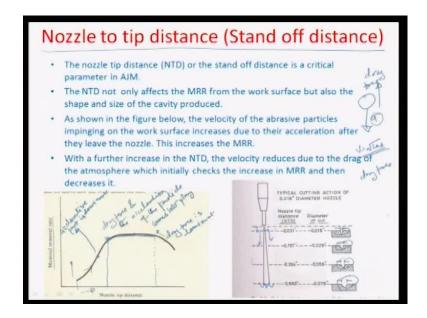
So, the acceleration is going to take this particle to a higher velocity of the distance that, you are allowing it to move this more. As you know v square minus u square is equal to 2 as keeping acceleration constant the velocity at u equal to or initial velocity equal to 0. The final velocity that you can achieve is really proportional to the root of in the distance.
