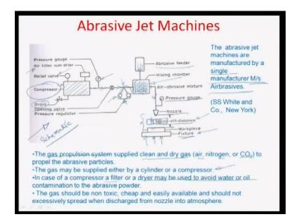
So, typically all these abrasive jet machines are manufactured by these company called Airbrasives in Newyork. And they are probably one of the single manufacturers for this particular system. If you look at the details of the system here, this schematic is very well illustrative of what all components go into abrasive jet machines.
