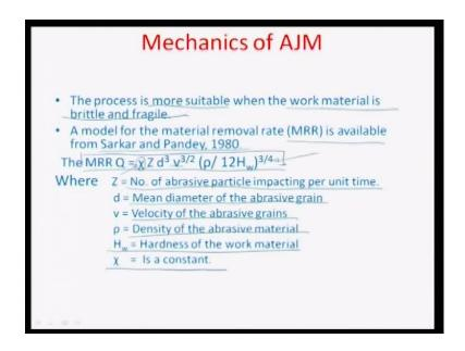
So, basically it is a fracture by fracture which would happen in succession for a cavity to be created within the work piece. So, as you can see here the wear particle here is carried away by, the flowing air or gas in this particular illustration shown. So, if you look at the process more closely. It is more suitable when the work material is actually brittle or fragile because then the it automatically promotes the process of brittle fracture.
