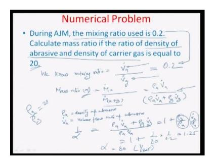
And I will just like to show you 1 or 2 example problems, where we calculate this. So, during an AJM process for example, the mixing ratio is that is used 0.2 and I have to calculate, in the mass ratio of the ratio of density of the abrasive and density of the carrier gas as is given, it is equal to 20. So, here we know the mixing ratio already from
