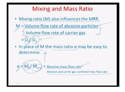
So, I already discussed in great details about the mixing ratio and also the influences, on the material removal rate of the process and. So, the mixing ratio has I earlier defined is known by this quantity here, the volume flow rate of abrasive particles by the volume flow rate of the carrier gas and. So, if you are loading more than this mixing ratio goes up and vice versa.
