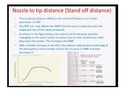
So, normally for I mean; sort of standard operations of the industry cross sectional area of the r f s is circular in nature. Or it can be sometimes rectangular. And the r f s can have an area of about 52 200 microns or so in terms of the small you know cross section through which, the velocity the jet actually emanates out into work piece. So, these are some of the important aspects of the AJM process.
