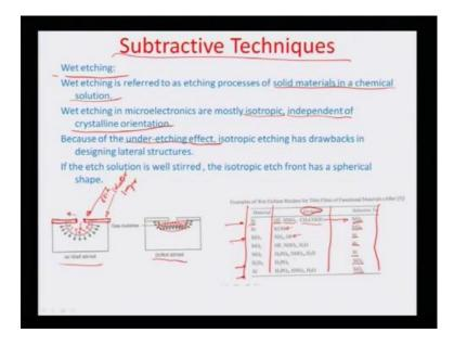
And for doing that, I would like to highlight this etching technique, subtractive techniques. So, what is really etching? Etching is the, you know is referred wet, etching can be dry as well as wet. And let us first see what wet etching is. So, wet etching is really a process, where solid materials can be immersed in a chemical solution, and the solution can displace atoms or molecules from the surface of this material because of certain chemistry is in reaction.
