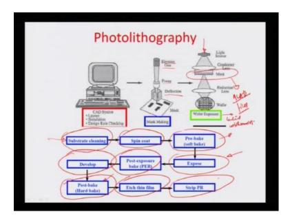
So, if you look at photolithography in a step by step manner, we lead is illustrated here as an example. So, you have a mask surface as you can see here, this is the mask. And this mask is actually made more or less using the power of A cad or auto cad files, and they
