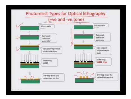
So, typically there are two different kinds of resists which exist. And this particular illustration here, kind of shows what would be the role of the two different kind of resists. One is the positive tone resist and other is a negative tone resist.
