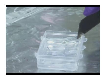
So after this whole heating process is carried out for about 85 to 90 degrees for about close to 45 minutes to 1 hour. You have a box kept here, so this was labeled in this particular leveling plate inside the oven, and you have quite uniform layer of PDMS which is solidified on the top of this these structures here, which is made up of the laser machine PMMA surface.
