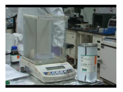
So here you now prepare the PDMS mix as in the next step, so you use that same process of measuring by weight. And you know there is a mould box again a sacrificial mould box being used. And you will be using this the commercial brand available for PDMS by you know mixing
