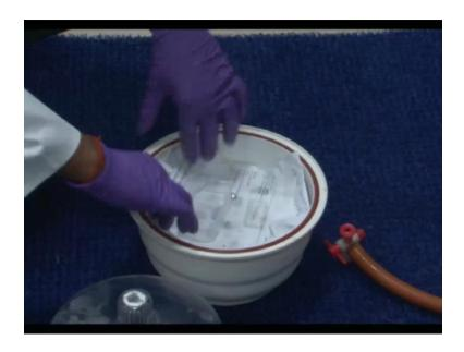
So it is becomes glassy. So now you can actually put the glassy pattern, inside the decicator and heat cured this with sorry the and chemically treat this with HMDS- hexamethyl diasolusin, so that again the glassy surface of the PDMS that has been created can be coated with suitable fluidic, layer.
