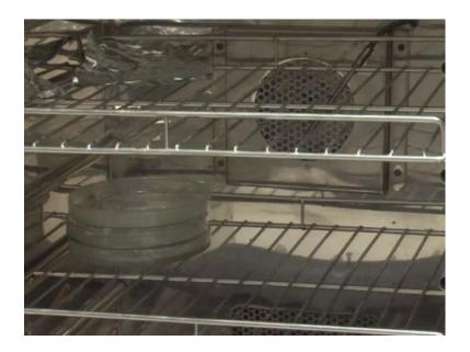
In the mean time you also should check the conditions of this gravity fact convection oven which has been sort of now (( )) installed about eighty five degrees Celsius, and all the way you normally.
