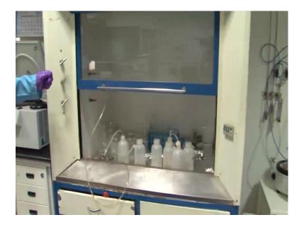
Hood something like this where you can break open the cape of the h m d s, and transport the bottle all the way into the desiccator, and then vacuum air head before doing that you ensure that you put this into the desiccators. So, that the environment given by the vapours sort of dust a preliminary treatment of this surface by giving small coating on the surface. So, as you can see now the processing of the while (()) is done.
