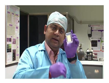
Now, looks, and you can see,, because of the tape it does not go anywhere, and when you pour something which is liquid in it there is always bawan (()) forces through which the mold might come up unless have been fixed. So, this we did for ensuring that the mold does not flowed up,, because of the bawancy (()) of the liquid in any event.
