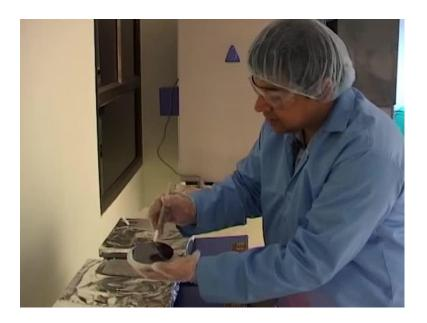
So, what will do is will go ahead and pull out the resists, now the resists could it wafer now. Again, the same precautions need to be followed, you need to hold the resist from a very, you know small corner here. And then, slowly put it over the surface that we want to mean want to put it. So, I am going to now transfer this resist coated wafer on to this particular surface. It is almost a good a idea to actually coat the headed surf or it hold the headed surface at room temperature.
