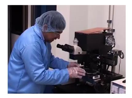
So, what I am going to do is to actually align this mask in it is space here and slowly. So, there are two slogs really for that purpose. And I am going to actually make it face down. So therefore, the chromium side has to be facing the wafer surface. So, which is actually given by this dark brown region of the mask. So, I slowly put it inside the mask holder.
