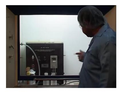
So, let us look at the components one by one. This right here is one of the fundamental component used in such a laboratory. It is known as the fume hood, essentially it provide the class 1000 clean space or clean area, which is just underneath of behind the particular
