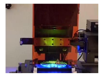
So, I am going to now actually turn on the exposure light. And as you see here, the moment I turn it on, the timer clock has started. And there the light, the UV light is now falling sharply on to the wafer. And essentially, this is the time reading here says, that is rapidly reaching 22 second mark, that we had set before. On the moment that is done, this light will go off, the explores light will go off.
