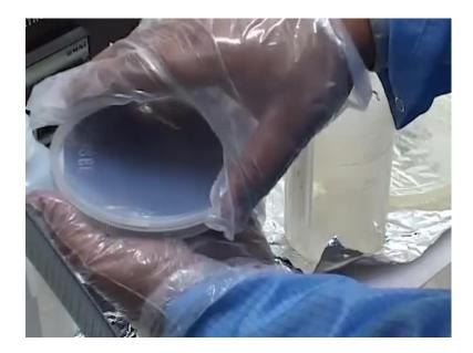
And that way we have a completely dehydrated surface, we need to cover it at this stage. Because, the moment we move it out of this clean area. It can again become dusted, and the contamination of the surface may happen. So, this is how the piranha cleaning process of the wafer is done. So, basically what we do now is to take this wafer, that we just made super clean using piranha process; and take it to a oven.
