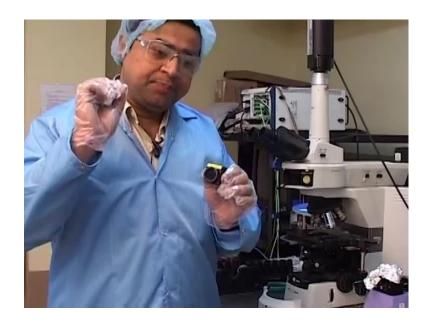
These cube have you know two they are cubes which have two filters essentially what are filters? Filters are essentially pieces of glasses, which and the sign to the cut off certain frequencies. And let certain frequencies of flied go blasted. So, in this particular filter cube as you see there is a emission filter, which is a situated at the top there is an excitation filter, which is actually situated here.
