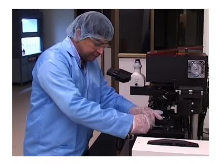
And essentially, you can actually now use the locking mechanism to ensure that, they firmly get locked over the wafer surface. So, what we do is now actually after mounting this properly, we need to actually bolt it firmly. So, we are going to actually use these set of screw heads to ensure. That there is a good contact between the holder, and it grips really on the surface. So, we are going to just ensure proper gripping of the holder, of the mask holder on to the surface of the stage.
