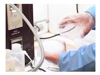
So, the first thing I am going to do, is to actually un load a wafer from it is box. And make a separate container, take a separate container on wafer box. And transfer this wafer, as you are seeing here, this right here really is wafer box, which is meant for containing a single wafer. For micro fabrication, it is very important that specially when the wafer of moving between workstations, we need to cover the wafer adequately.
