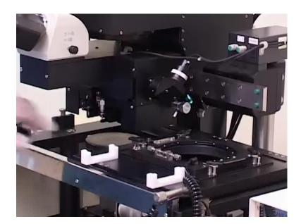
So, here we have something called a mask holder which is actually this region here. The mask is really setting on the top of on the bottom side of the surface of this particular holder. And it is actually facing the wafer which would be placing somewhere here. This
