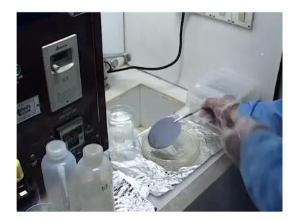
So, these as you see are now Teflon coated, these two is a soft tips which are coated with Teflon. Or they can be complete Teflon tweezers, which we can use. So, what we are go going to do is to provide a normal rinsing, using distinct water. As you can see here, which is resting in the ((Refer Time: 17:49)) of this particular piranha clean wafer sample. And then, this would be followed by another wash of DI, DI and I use to water. So, that it gives a super clean, surface on the wafer.
