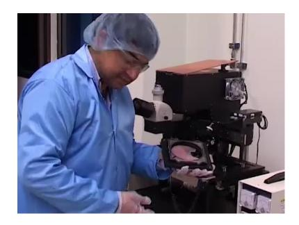
And essentially, as you see this really is a surface which holds, this particular hard mask. And then there is a stand for this application or this mask loading. You have to put it right in that particular spot, it is like a jug. And it ensures that there is no unnecessary toppling or falling down of the mask holder.
