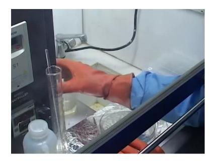
And so what we now do is essentially take this piranha, what we have prepare. And then, pour it over silicon wafer, which will be keeping in this particular petri dish separately. So, what we do is essentially, we take our wafer, silicon wafer and open this. And clean, in order to clean this wafer, we put this wafer back over the petri dish here.
