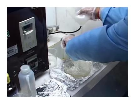
And slowly rinse it on the surface of this particular wafer. As you can see here, this actually a spot bottle, which is sporting away the DI water on the top of the silicon wafer. So, essentially after completely rinsing it, you basically try to just change it is holding location, to a different area. So, that you can rinse of the acid in the particular area, where it was held before, and this way you can clean whole sample.
