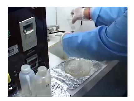
So, what we do is to basically pull it out very carefully, because essentially this is all acid coated now one has to be very careful. And then, hold this over this edge and rinse it inside this with water. And rinse it on both side, as you can see all the water should typically go. And rinse all the acid of the surface of the silicon wafer.
