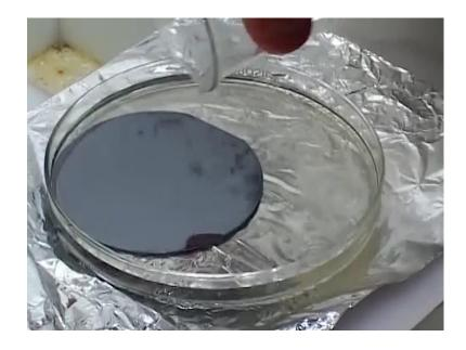
As you can see here, we are putting the wafer in this petri dish. And once we pour the piranha, we can no longer use this metal tweezers for handling this wafer. So, will have another separate step 1 tweezers, for doing this wafer handling, once it is out of the piranha for washing and rinsing. So, now you slowly pour this chemical the piranha over this wafer. And it is extremely hot as you can see. And essentially, it also fumes as you pour it.
