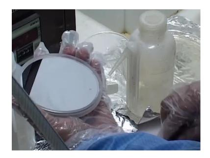
So, we put this sample, this clean sample back into the wafer box, as you can see. And then, will actually do a heat treatment of this particular wafer, so that it can get rid of all the water from the surface.
