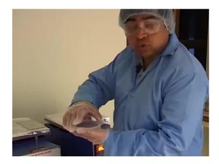
So, we are now ready after this temperature is close to the room temperature to do lithography on this particular wafer. So, essentially this is call the photolithography equipment. And this is used for explores of the resist to very characteristic frequency of light mostly in the u v area. Essentially, here what you do is to use something called a hard mask, which you can see here right here.
