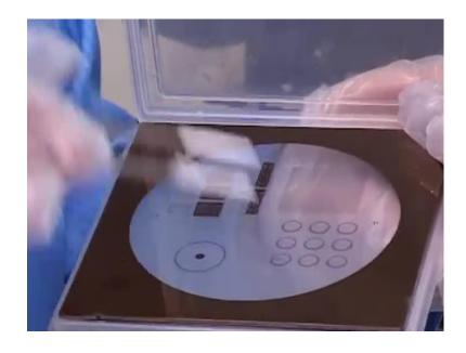
This is actually glass crow mask, where you can see very closely, if you look at some of these features really are at the microns scale. And these have been made using a laser etching in a film of crown, that in ((Refer Time: 47:02)) that this side, this particular side which has the coating really switch with the wafer being aligned with the wafer.
