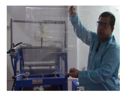
So you can see that two forms right here, this is the packaging of the four I laboratory, and this again is the packaging of that particular fuselage of the aircraft. We have just kept if for representational purposes, of the idea here is that very small features can also be very well formed with this particular method.
