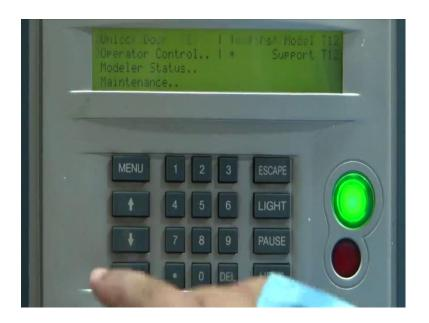
And then, basically try to prepare the stage for this particular run. So, what we are wanted to do is, to sort of go into this operator control, which is the second option here which in can use the cursor key to go. And then, enter on this operator control which takes me in to another menu, sub menu which say unlock door, load, unload so and so forth. So, I am going to again enter because, there is an unlock door option which is there.
