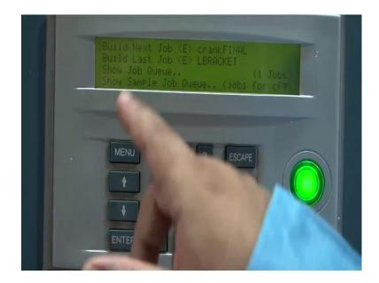
So, once we do that, we can see that we are talking about build next job. And then, they are saying crank final. So, this is the job which has been queued to the machine. I am going to build this job now. And the movement I press the menu key here, you will see that first, the stage would go all the way to the initial position.
