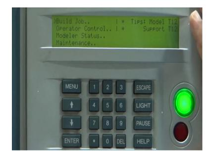
Though, the controller here as you are seen for the r p of the machine, after homing of the x y z as happened. Stage has happened shows a lot of options like build job, operator control, model status, maintenance, so on and so forth. Each of this has certain meaning. And I will describe these along the way I do the machining process. However, once we want to just actually, first clear the stage with existing whatever is lying inside from the last run.
