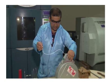
You can see, this is a wire roll. And this is what the basic raw material comes as. And this wire is fed from a very small nozzle, which actually is able to move in a x, y plane with the information that, it would have the coordinate positioned information, which we should have from the cad file. So, suppose if, now there is a sectioned layer of such a complex part, I showed you a part can be as complex as this.
