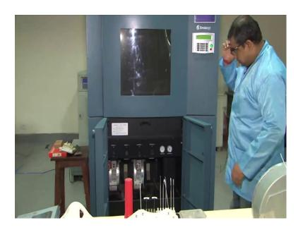
So, as you can see here, there are two parts basically of the machine. One is the controller part and also the material feeding part. The rolls are now, currently in position and they are fed in the system. And the controller, here is actually indicating several different aspects like, what is the support material? What is the model?
