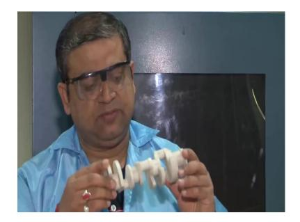
This is the crank share of an automotive. You can see the design and you can look in to the kind of complexity, which is involved in designing such processes. Typically, this is used in the automotive industry. And the way you generated is, using forming processes, but here you basically depositing and making a scaled prototype or a model. Through, which you can probably formulate the next step, which can be used for a DI manufacturing for that forming process to happen.
