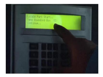
So, if you go back to this particular controller here, you see there is an option which says demo bounding box. All it means is that, when I am going to press this demo bounding box, ((Refer Time: 42:06)) It will show the domain within which the printing has to be done on the surface of the 3D printer. So, I am going to just select this particular operation here, do the enter... And you can see that there is domain tool path has gone inside.
