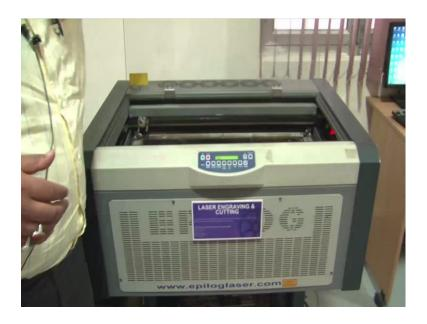
So, today we have with us this small laser, and graving, and cutting system which is from company called epilog this tool is working on the principle of a small ton micron spot of laser which scans, and raster the surface a that is grading the engravement or the formulation of the microchannel within soft, and hard polymeric material. This is a the
