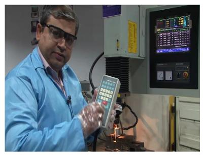
So, in fact, there is this punching box which is there in this machine, for doing the various, punching the various commands. And, this right here, the screen is what you can see is the display of the controller, so this is actually the controller unit which will do the servo controller action. And here, what we can do is, by standing at a little bit distance we can actually do this controlling.
