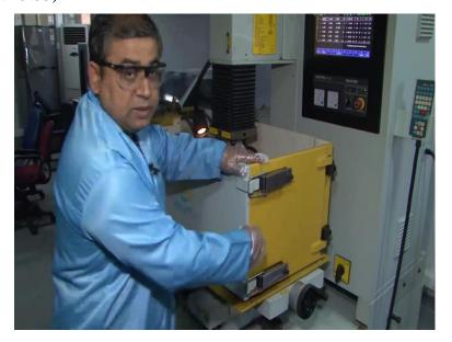
So, you have to just open this clamps here. And, just declamp this, so that we can open up the box in both the cases. And, this is how, so you can actually open this cover as well as this, and then the whole idea is to be able to extract this work piece from this gig here.
