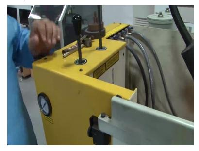
And then, what you do is the following. You basically use this leaver and try to close the valve, so that the e d m oil in the tank can now start raising. You can see that the oil level is now started to
