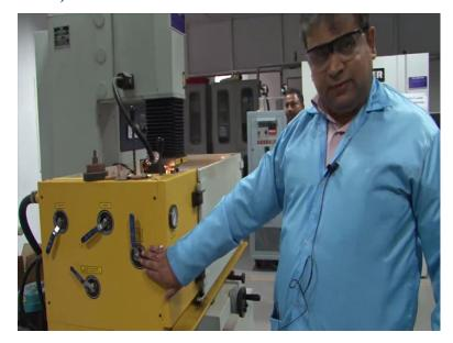
Now, we will go for the next step which is filling of this tank, beyond which will start the machining. So, here now, we would like to give a little bit of illustration about the dielectric dispensing system associated with this machine. And, for doing that, what is important is that, there are different valves on this machine as you can see which perform different from functions.
