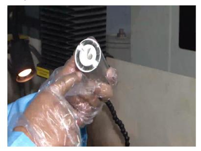
So, I just like to show you, how the e d m process has been done on this particular work piece. And, I just kept up the oil, and you can see that shape that we were indenting to was that, comma shape at object of which electrode was, is being now printed on to the surface. And, this can go upto, all the way from 100 microns to, almost about to few tens of millimeters, and that is the advantage behind e d m, that it can go upto any extent.
