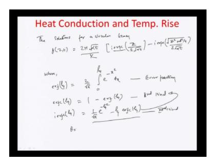
So, if we assume this to be the new boundary conditions the solution that would emerge to this equation for a circular beam they come equal to theta z t equals to twice h root of alpha t by k error function of the third kind z by twice root of alpha t minus same again times root of square of z plus d square by four divided by twice root of alpha t.
