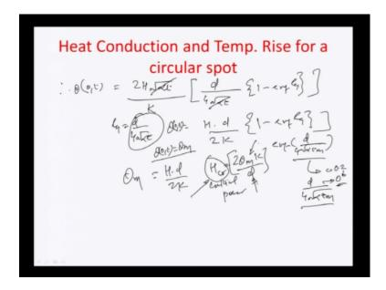
How we have zeta on the surface corresponding to z equal to zero at any function as a function of time t twice a h route of alpha t this is the beta value mind you divided by k times of now we have b by four root alpha t times of again one minus error function of zeta, and zeta is d by four root alpha t.
