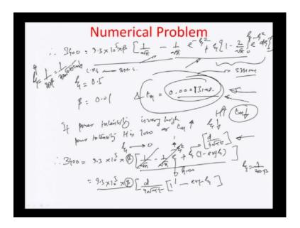
The solution of this equation thirty four hundred equals nine point three ten to the power of five times beta by one by root of pi minus one by root of pi e to the power of minus zeta square plus zeta times of one minus twice by root of pi integrate zero to zeta e to the power of minus zeta square d zeta this comes out to be corresponding to a zeta value of zero point five a beta of zero zero on, and time of machining zero point zero zero zero seven three seconds. So, it is a one three seconds.
