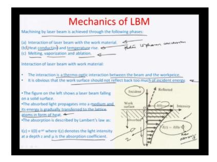
So, machining by laser beam is typically achieved by the following phases phase one is interaction of laser beam with the work material there is a photon to phonon conversion which rises the local temparature, and energy, and there is of course, heat conduction beacause of a sudden temparature gradian which is produced from the central of the beam to the side of the beam, and sudden rise of the central of the beam temparature, and there as of course, there is melting viporisation.
