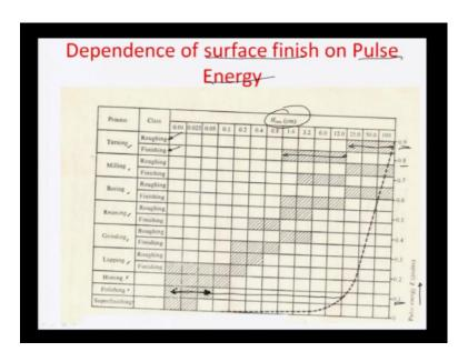
So, let us look now at the a more dependable relationship between in surface finish on pulse energy is illustrated in this process, here an you can see this spark energy on the right y access here in joules for the various operations a like electro discharge turning, and electro discharge milling boring reaming grinding lapping honing polishing super
