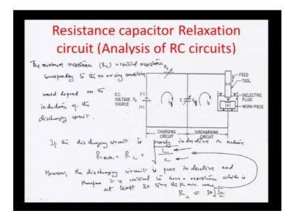
So, that minimum resistance r c that will result in a control of the process without the formation of any arking a such is known as the critical resistance for this particular circuit an. So, then the critical value of resistance corresponding to the no arking condition.
