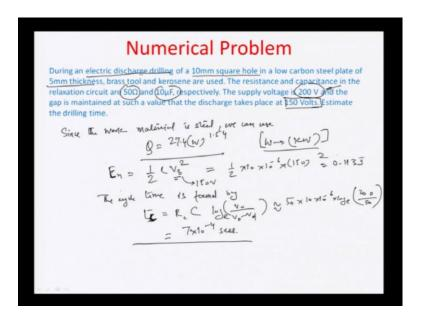
So, do an numerical problem based on that as illustrated here that in electric discharge drilling processes of a ten mm square hole in a low carbon steel plate of thickness of five mm brass tool, and kerosene are used as kerosene is dielectric brass is tool the resistance, and capacitance of the relaxation circuit that have been designed the given a fifty ohms, and ten micro respectively, and it also indicating or or it is also indicator.
