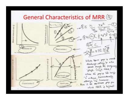
So, let us now look at some of the other important accepts some of the machine in trends with the different parameters that we have discuss. So, far. So, here a in this particulars slides we are illustrating in variation of the material removal rate q with respect would a parameter like the resistance of the charging circuit the mean current i, and this particular
