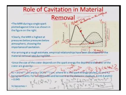
So, let us a look at the role of cavitation in material removal in the e c m process a refer to this particular figure here it is between pressure of the zone of the spark which is plot at on this y one access, and the material removal rate during a spark cycle queue is plot at on this y two access with time scale on the x access.
