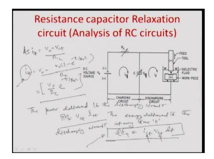
As i c t is actually to v zero minus v c t by r c how we can find this out. So, we already have the value of v c t from the previous equation as v zero one minus e to the power of minus t by r c c by r c, and therefore, a how we can write this down as v zero by r c e to the power of minus t by r c c. So, that is the value of the current in time.
