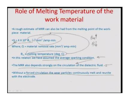
So, that relationship has also been defined in literature as if theta m were the melting temperature a in degree celsius of the material there the amount of material removal rate
